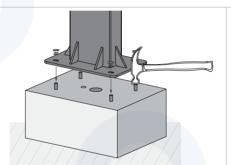
2) Install expansion bolts in the base mounting holes. Fix the column on the concrete platform with expansion bolts(x4).
