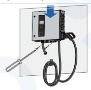
2) Place charger onto bracket. Align the back chassis of the charger with the corresponding slot on the bracket. Slowly slide down the charger until it sits firmly on the bracket. Fasten two screws from the bottom.
