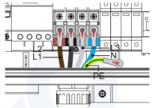
3) Pass the power cable through the bigger cable gland, crimp power terminal from the end of the power cable to be connected to the internal circuit breaker. Connect the ground wire(PE), neutral wire(N) and each phase(L) to the AC input configuration board, Connect the Ethernet cable to the motherboard via a PG connector.
