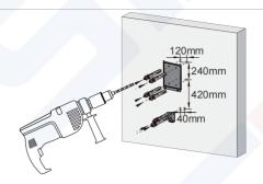
1) Use the bracket and hook to mark drill holes, Mount bracket and hook onto the wall. Use the expansion bolts in the accessory kit or choose proper mounting screws for different types of wall. Adrilling machine might be needed for certain conditions.
