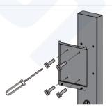
3) Install the bracket on the column.
