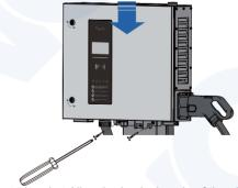
4) Place charger onto bracket. Align the back chassis of the charger with the corresponding slot on the bracket. Slowly slide down the charger until it sits firmly on the bracket. Fasten two screws from the bottom.
