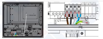
5) Pass the power cable through the bigger cable gland, crimp power terminal from the end of the power cable to be connected to the internal circuit breaker. Connect the ground wire(PE), neutral wire(N) and each phase(L) to the AC input configuration board, Connect the Ethernet cable to the motherboard via a PG connector.
