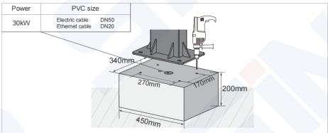
1) Make concrete platform, mark the holes position of installation column and drill holes.
